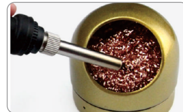
The steel wire has moderate hardness and does not hurt the iron head
