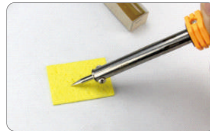
3.Clean soldering iron tip impurities
