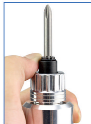
2.LOWER THE SCREWDRIVER HEAD AND ALIGN IT WITH THE DETENT
