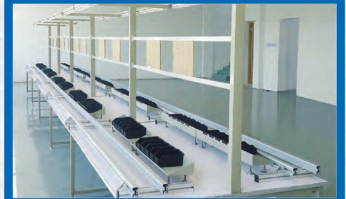
Double-sided non-powered insertion line
