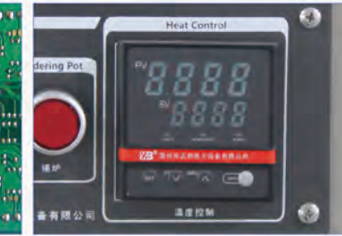
PID Intelligent Temperature Control
