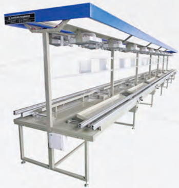
Automatic insertion line
