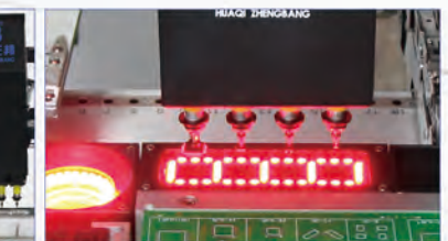
Four sets of fast recognition cameras
