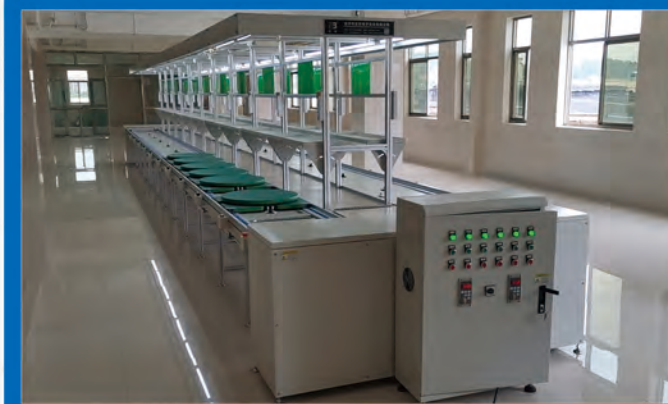
Horizontal loop high-speed chain assembly line
