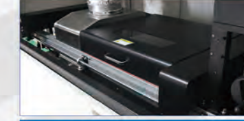
Preheating System Ensure even and sufficient preheating of the PCB board surface The temperature control method adopts PID+SRR closed-loop control
