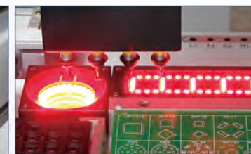
CCD high-definition recognition camera
