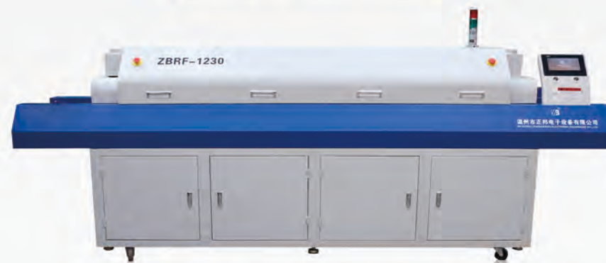
Twelve temperature zone Hot Air Reflow Soldering
