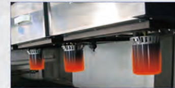
Using high-temperature long axis fans
