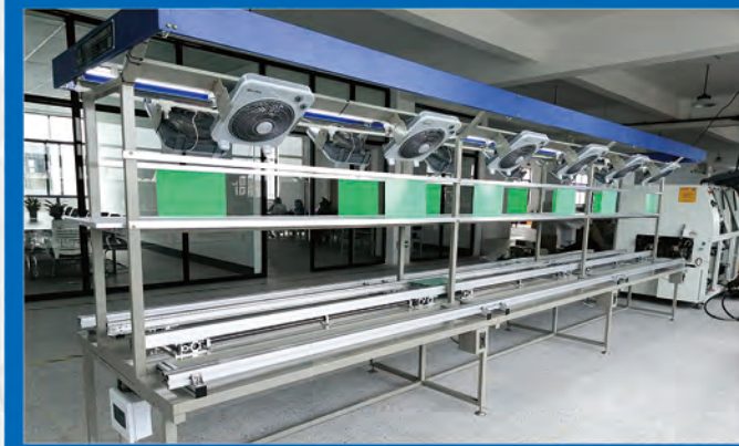
Double-sided automatic insertion line
